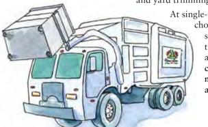
At single-family homes, hauling companies may choose to collect garbage and recyclables in separate trucks or in a single split-body truck that has a divider to keep garbage and recyclables separate. Regardless of the collection method, garbage and recycling materials are never mixed in the trucks or at the facilities where they are taken.
